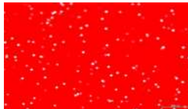
Figure 8 Photomicrographs for the revelation of the alpha particle tracks in LR-115 detector for Am-241 source
