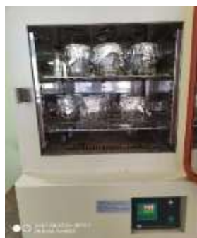
Figure 6 Chemical etching of the detectors in an oven
